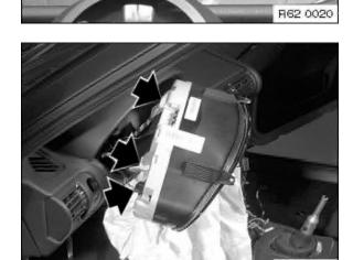
Push levers on connectors forward and take out connectors.
